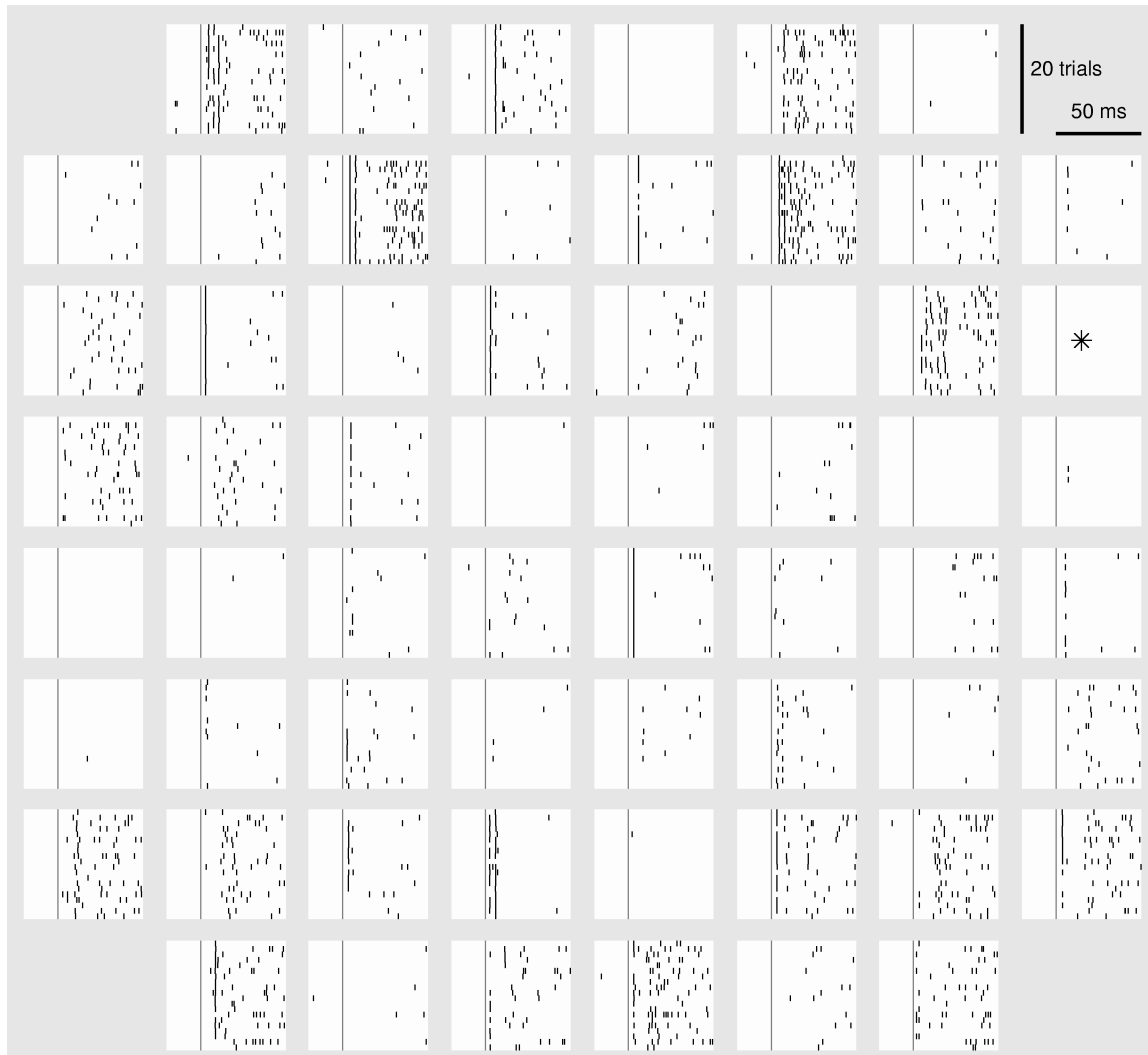
Figure 6.5: Array-wide responses to stimulation. Each graph shows the responses on one electrode, represented according to the geometry of the array. The stimuli were delivered to the marked electrode. Vertical line indicates time of stimulation. Spikes were detected after artifact suppression (Wagenaar and Potter, 2002); TTX control confirmed the biological origin of all detected spikes.
