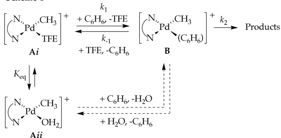
$$-\frac{d[\text{Pd}]_{\text{T}}}{dt} = k_{\text{obs}}[\text{Pd}]_{\text{T}} = \frac{k_2}{k_{-1}[\text{TFE}] + k_2} \cdot \frac{k_1[\text{TFE}][\text{C}_6\text{H}_6][\text{Pd}]_{\text{T}}}{[\text{TFE}] + K_{\text{eq}}[\text{H}_2\text{O}]}$$
