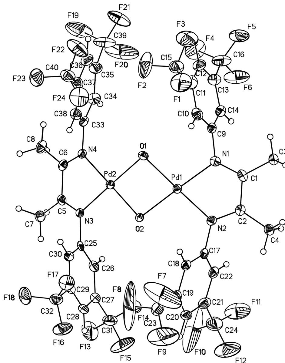
**Figure 2.** Molecular structure of **5b** with 50% probability ellipsoids. Hydrogen atoms and anions have been omitted. Selected bond distances (Å) and angles (deg) are as follows: Pd1–Pd2 = 2.9706, Pd1–N1 = 1.993(3), Pd1–N2 = 2.000(3), Pd1–O1 = 2.025(3), Pd1–O2 = 2.022(3), Pd2–N3 = 1.987(3), Pd2–N4 = 1.991(3), Pd2–O1 = 2.022(3), Pd2–O2 = 2.025(2), N1–Pd1–N2 = 79.03(13), N1–Pd1–O2 = 177.05(12), N1–Pd1–O1 = 99.60(12), Pd1–O1–Pd2 = 94.44(11), Pd1–O2–Pd2 = 94.45(11).
