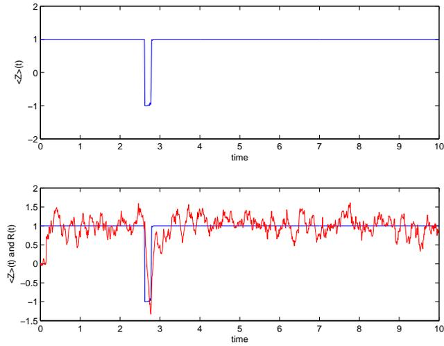
Figure 5.1: A sample trajectory of the one qubit "code" with feedback. The top graph just shows the expectation value of  $Z$ , and the bottom graph shows expectation value of  $Z$  and the filtered signal  $R(t)$ .
