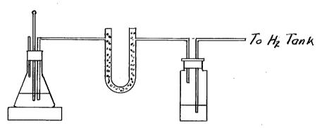
The flask containing the oil and catalyst to be tested was put on an elect ric hot-plate and heated to a temperature of 180°C (temperature of maximum hydrogenation). Hydrogen was then bubbled thru the oil from the cylinder until the ballon was partially filled and assumed the position shown by the dotted lines. The flask was then shaken and the ballon would collapse, due to the hydrogen being absorbed by the oil, if the catalyst were active.
